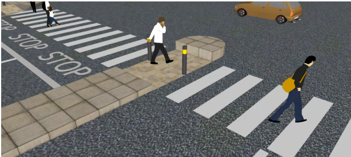
Figure 39 General Aspects of Safety Design - lane markings, signage, traffic-calming, pedestrian crossings and median dividers.(EMBARQ India 2014)
