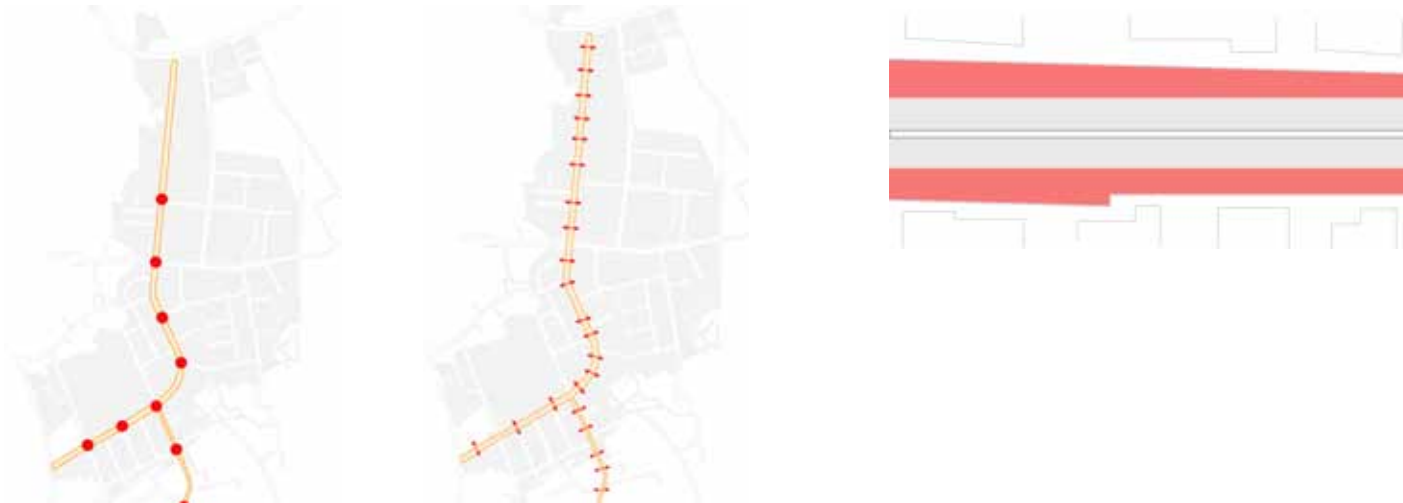
Figure 32 (left and middle) Raised intersections and pedestrian crossings; (right) Consistent carriageway & reduced lane widths, Source: EMBARQ India
