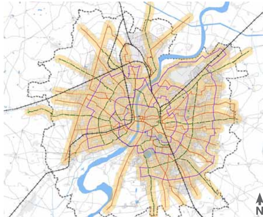
Figure 30 Trunk (BRTS) and feeder bus zone of influence in Ahmedabad, Source: CEPT University
